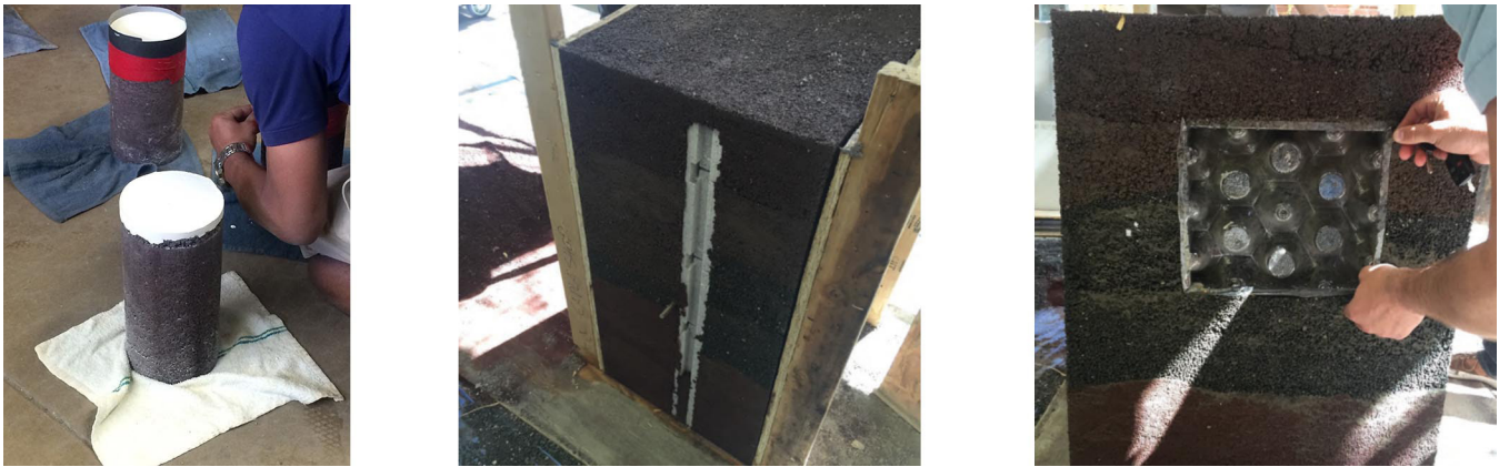
Figure 1. Scoria test cylinders and full-scale mock-ups. Photos by author.
